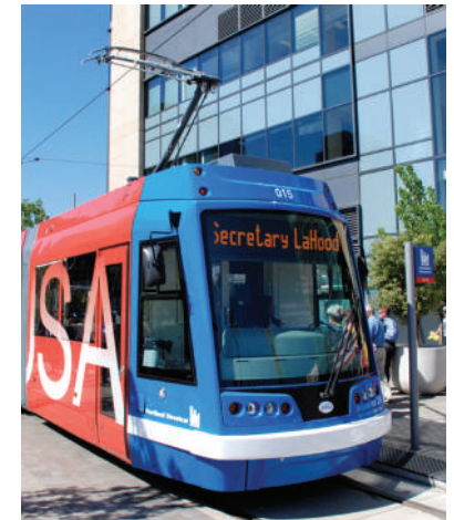
A streetcar from the Portland Streetcar line: streetcars similar to this model are able to climb hills that have a 9% grade
