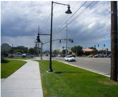
New street and pedestrian lighting found near Highland Dr: The lights are the first pedestrian lights found on the street. A majority of the street is lined with cobra lights directed onto the roadway, so much of the sidewalks remain dark
