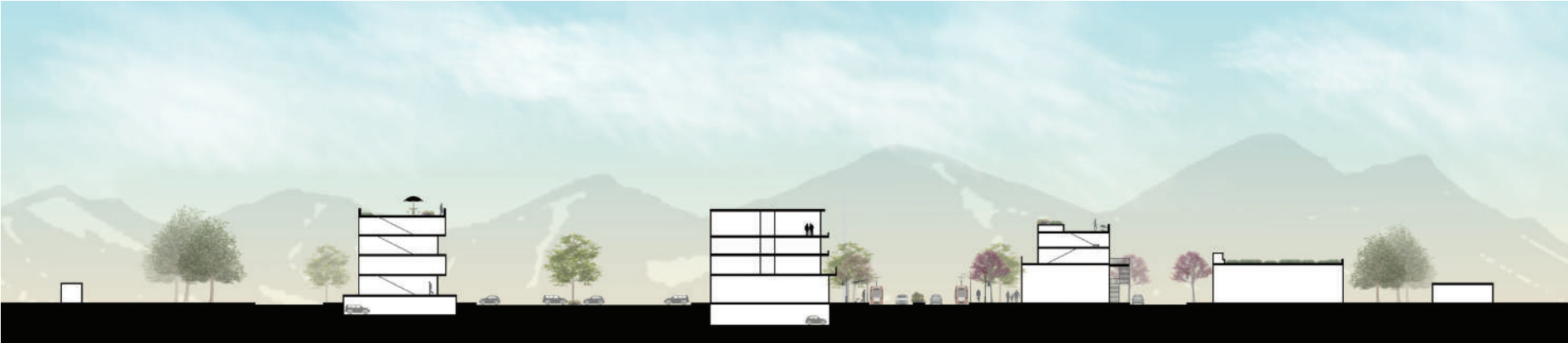
Section of the infill and redevelopment of the Cottonwood Mall area: mixed-use retail and residential units will be built near the street in front of the strip mall. In time the mall will be removed for additional mixed-use buildings
