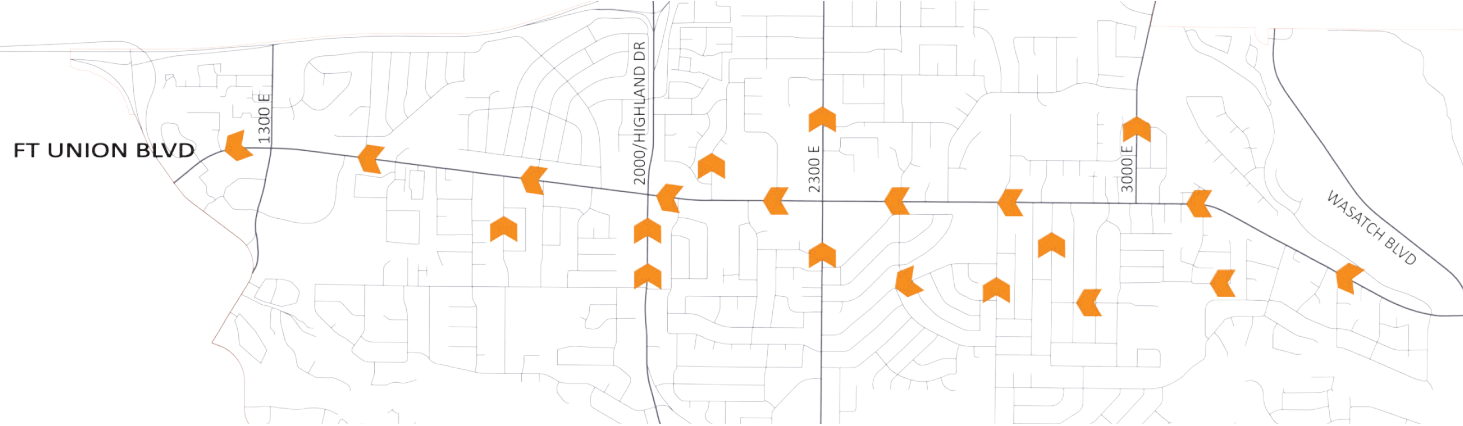
Drainage map of Fort Union Blvd: shows the waters movement from the canyon as it travels towards the Great Salt Lake. The natural flow provides Fort Union Blvd with the opportunity to better manage the water as it travels west by such practices as bioswales and permeable paving
