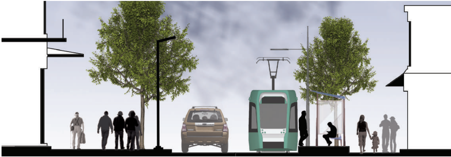
A typical street section showing through a one-way street: The raised platform for loading dissipates into space for on-street parking in this configuration. The narrow one way streets allow for large sidewalks for pedestrians
