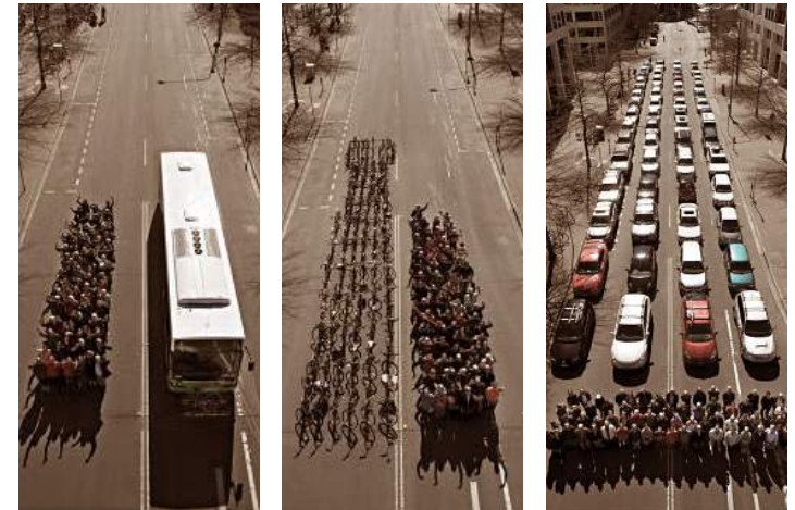
A visual comparison: the same number of people that fit in a city bus as compared to cars and bicycles and the space required for each
