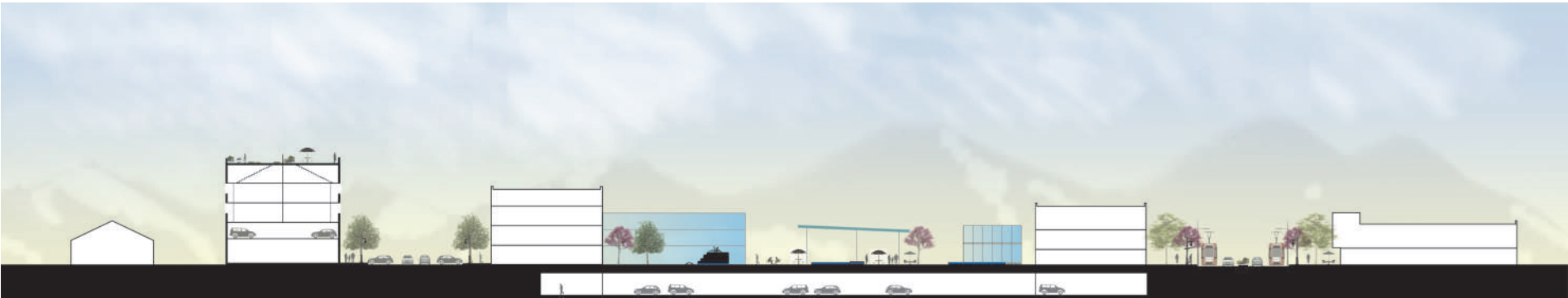
Section of the infill and redevelopment of the Whole Food's parking lot: the new design places parking underground to allow for new buildings and a new plaza space for dining and gathering. The location of section cut lines can be viewed on the illustrative plan of the design proposal
